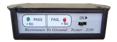
The **grounding** of ESD protective equipment is used to reduce the chance of damage to susceptible parts and assemblies resulting from ESD. The first step in ensuring that everything is at the same electrical potential is to ground all components to the same electrical ground point. This point is called the **common point ground** and is defined by **ANSI EOS/ESD/S6.1** as a system or method for connecting two or more grounding conductors to the same electrical potential.
